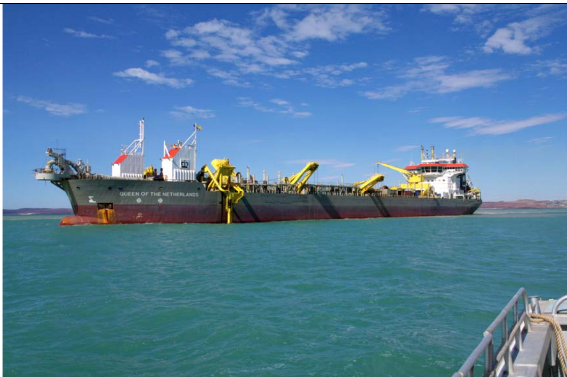
Plate 4: Queen of the Netherlands completing channel and berth pocket dredging works, May 2010.
